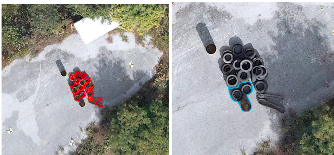
Figure 6. Left: Examples of ground truth labels with tyres. Right: Examples of the TextSAM model mask that includes both a true positive and a false positive, considered a true positive.
