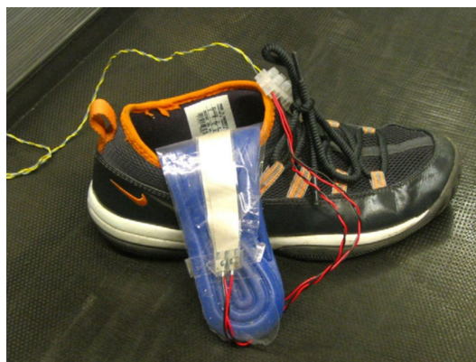
Fig. 6 Prototype of a piezoelectric film inserted in a shoe. Reprinted with permission from [126]. Copyright Elsevier, 2006
