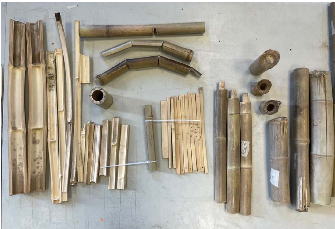
Fig. 6 material experimentation on the lower part of the bamboo culm, a secondary by-product of harvesting
