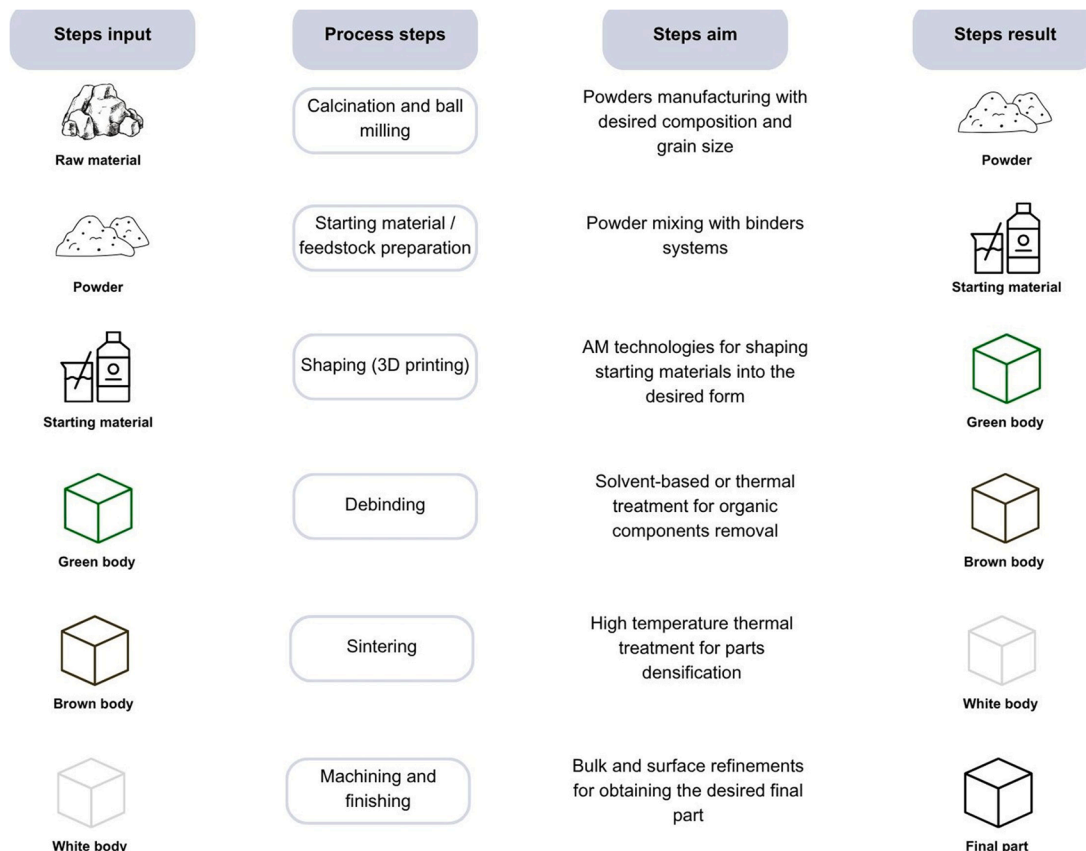
Fig. 1. General process chain in fabrication of ceramic objects, with AM technologies as shaping methodology (CerAM).
