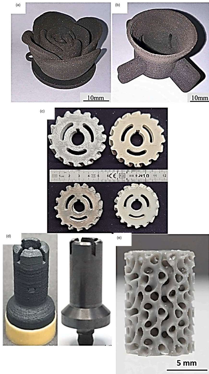
Fig. 3. Example of CerAM printed objects, through different technologies: (a) and (b) a rose and an impeller-like structure in \text{Al}_2\text{O}_3 fabricated through CerAM BJT; (c) gears in SiC (on the left) and \text{Si}_3\text{N}_4 (on the right) fabricated through CerAM MEX (FFF), before and after sintering; (d) a ceramic plasma plug fabricated through CerAM MMJ; (e) triple periodic minimal surfaces component in \text{Si}_3\text{N}_4 fabricated through CerAM VPP. (a) and (b) are reprinted from Additive manufacturing, vol. 79, Z. Yang, L. Yang, P. Wang, Z. Peng, Y. Niu, W. Jiang, Z. Fan, "Effect of sintering aid combined vacuum infiltration on the properties of \text{Al}_2\text{O}_3 -based ceramics via binder jetting", 2024, with permission from Elsevier [17]. (c) is reprinted from [18]. (d) is reprinted from [19]. (e) is reprinted from Journal of the European Ceramic Society, vol. 43, issue 2, E. Schwarzer-Fischer, E. Zschippang, W. Kunz, C. Koplin, Y. M. Löw, U. Scheithauer, A. Michaelis, "CerAMufacturing of silicon nitride by using lithography-based ceramic vat photopolymerization (CerAM VPP)", 321–331, 2023, with permission from Elsevier [20].
