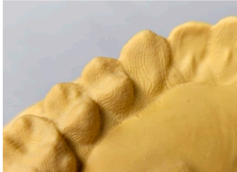
Figure 2. Dentations of the inner surface of the aligner. Note the ability to detect surface striations of the aligner due to the 3D printing process.
