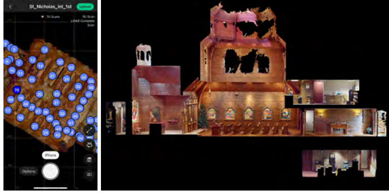
Fig. 3. Mobile application interface to control Matterport Scanner, screenshot showing 70 scanning locations in an S-shape route on the main floor. Section perspective of the aligned interior scans of the whole building.
