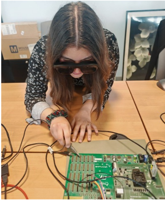
Fig. 6: User localizing a pin through ARBoard application running on XREAL Air 2 Ultra
