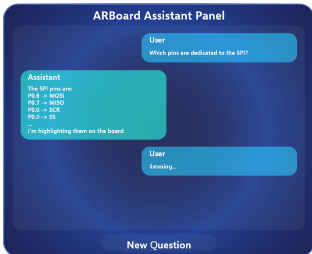
Fig. 5: ARBoard AI assistant answering technical questions and highlighting component on the physical board
