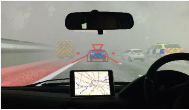
Fig. 9: AR-HUD interface for safety enhancement displaying icons with different colors depending on the distance, overlaid on every vehicle. Image adapted from [15].
