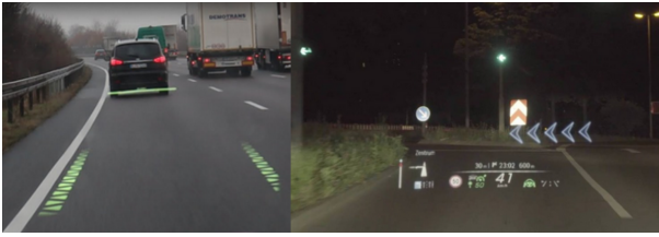
Fig. 5: Left : an example of AR-HUD from Volkswagen, highlighting the lane and the vehicle preceding; Right : AR-HUD interface from Mercedes, with chevrons indicating a left turn.
