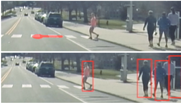
Fig. 8: Top : The virtual shadow ARGE indicates the direction of the pedestrian crossing the road as a shadow in front of their feet. Bottom : The red bounding boxes highlight the figure of every pedestrian on the curb and crossing the road. Images adapted from [163]
