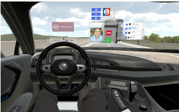
Fig. 11: Examples of GEs that support NDRTs on AVs. On the right of the HUD, we see several apps open (i.e., media player, video call app, and a social media comments section), while on the left a TOR request is displayed. Image adapted from [123].
