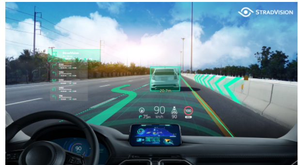
Fig. 1: AR-HUD concept by Stradvision [9] showing spatially registered warnings (maneuver suggestion, collision warnings) together with non-registered informational elements (navigation instruction, dashboard information).
