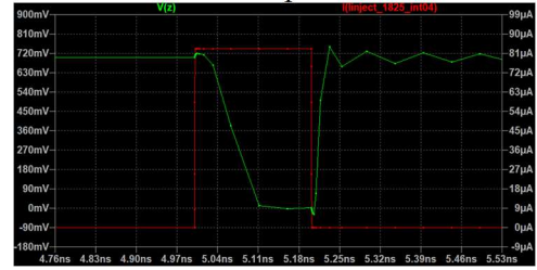
Fig. 7. An example of the injected pulse and triggered upset.
