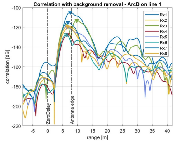
Fig. 11. RAAD response from all line for an arc occurring in the antenna
