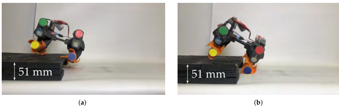
Figure 11. Lateral tipping associated with instability caused by unsynchronized wheels: (a) Three-spoke wheel at a height of 1.7R (51 mm). (b) Tapered three-spoke wheel at a height of 1.7R (51 mm).
