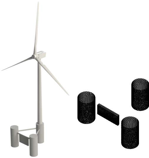
Fig. 1. Schematic representation of the analysed hybrid wind-wave energy converter (left), and corresponding hydrodynamic panel mesh used for the BEM analysis below the still water level (right).
