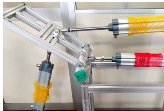
Figure 1b Some details of the current pelvis simulator.
