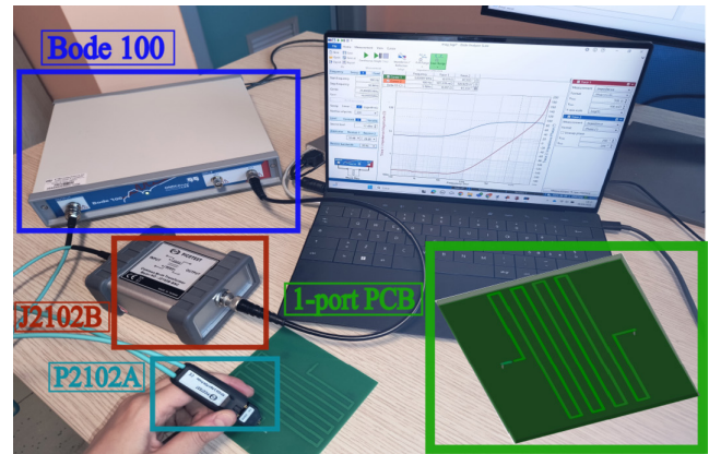
FIGURE 2 | Measurement setup with Bode 100 (and Rigol RSA 3030N) as VNA, J2102B Common Mode Transformer, two-port probe P2102A and PCB layout.
