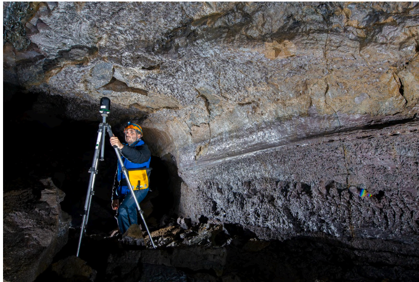
Dr. Riccardo Pozzobon mapping with a laser scanner the interior of a lava tube in Iceland. Marco Vattano with permission.
