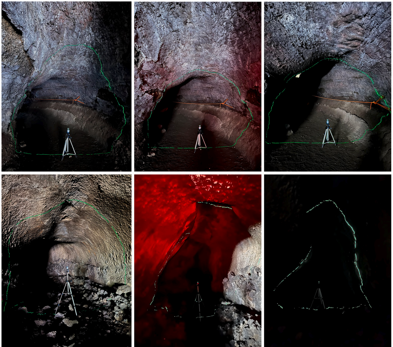
Fig. 3. Above: the Grotta dei Tre Livelli-KTM, upper branch, around 10 m from the entrance pit. Below: sections of the north-east upper branch of Grotta del Monte Intraleo, from the entrance through the dark areas of the caves. In both cases, it is possible to observe how the utilisation of a 360-laser level, in this case a Dexter 360 laser level, allows the creation of “real-time cross-sections” that describe very well the actual internal forms and shape transitions.
