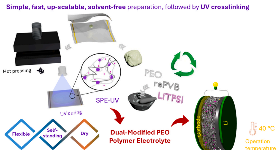
Fig. 1. Schematic illustration of the SPE-UV electrolyte preparation process.
