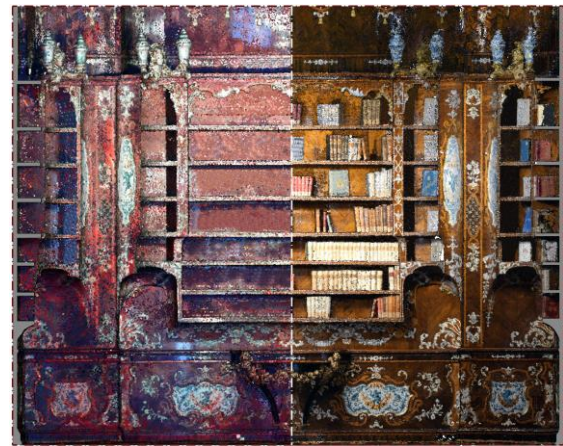
Figure 2: The front side of the library. On the left is the range-based data, and on the right is the point cloud from photogrammetry. (Editing: M. Russo)
