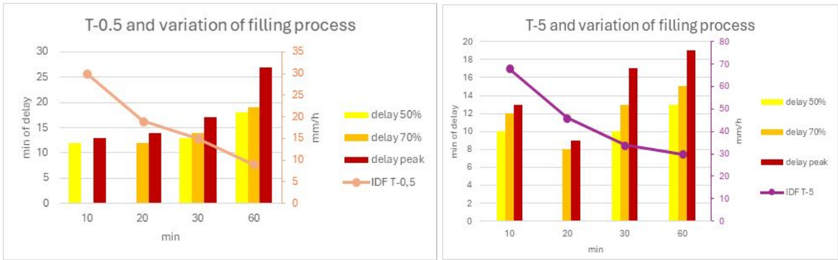
Figure 4. Variation of parameters for filling process over the IDF curves for 2 return periods a) T:0.5 year b) T:5 year.
