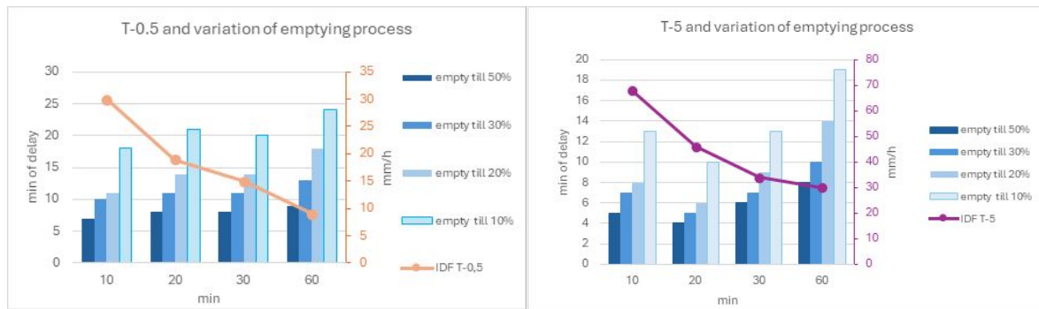
Figure 5. Variation of parameters for emptying process over the IDF curves for 2 return periods a) T:0.5 year b) T:5 year.
