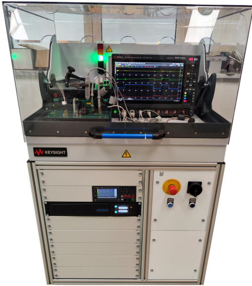
Fig. 1. Keysight PD1500A Double Pulse Test (DPT) system used for the high-precision characterization of 30 Infineon IMZ120R030M1H 30 mΩ CoolSiC 1200 V SiC trench MOSFETs.
