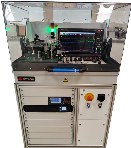
Fig. 1. Keysight PD1500A Double Pulse Test (DPT) system used for the high-precision characterization of 30 Infineon IMZ120R030M1H 30 mΩ CoolSiC 1200 V SiC trench MOSFETs.
