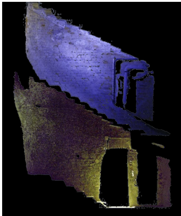
Figure 5. Point Cloud Section of Staircase (it is possible to notice the difference in radiometry due to light conditions).
