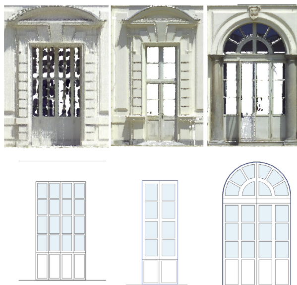
Figure 6. Examples of Door Types and Orthogonal Point Cloud Images (Top), Different Doors families (bottom).
