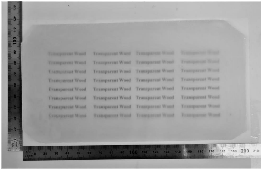
Figure 11. Scale-up demonstration of transparent birch wood infiltrated with melamine-formaldehyde resin. The sample was placed on top of printed paper. Reprinted from (Samanta et al., 2022) under CC-BY 4.0 License.
