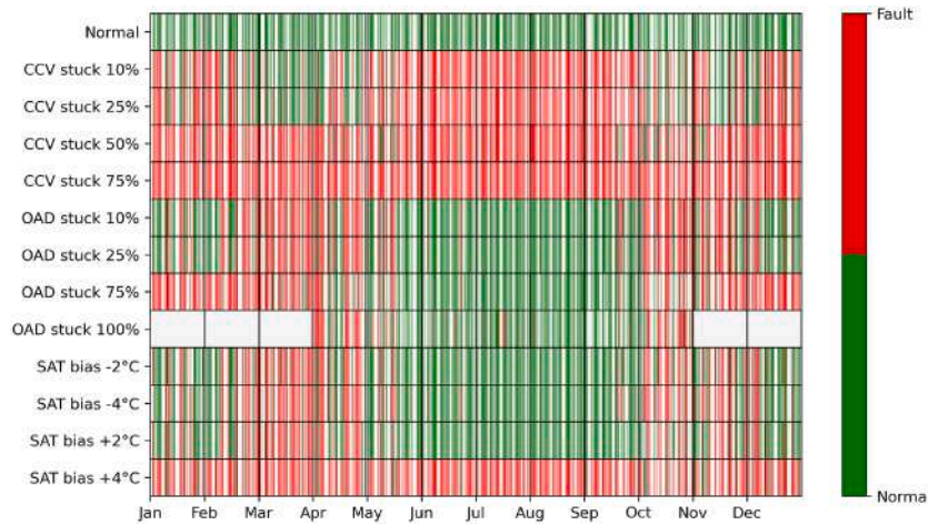
Fig. 7. Identification of Normal operation in Scenario 1 - Limited knowledge of the system.
