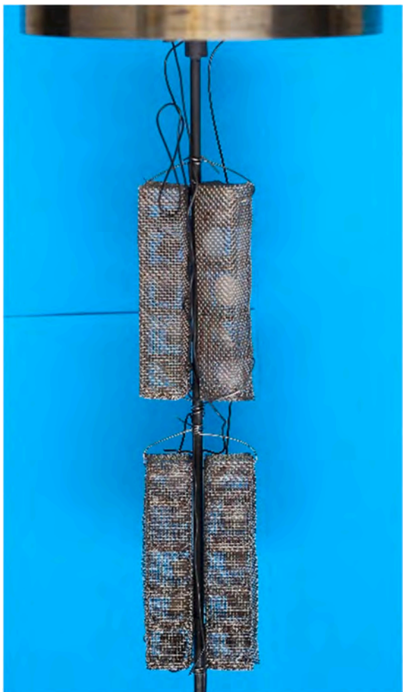
Fig. 3. Experimental arrangement of the test specimens for the PWR loop (CORTELINI, SCK•CEN).
