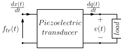
FIGURE 3. Two-port representation of the piezoelectric transducer.
