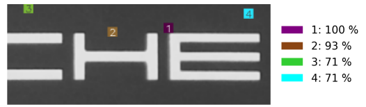
Fig. 13. Defect aggregation on 14 acquisitions of a brake caliper (SSIM threshold = 225/255, min cluster size = 15). Colors represent detected defects with respective occurrence rates.
