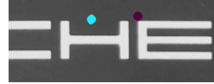
Fig. 7. DBSCAN result (similarity threshold = 210/255, min cluster size = 25). Two of the four SSIM-detected areas have been filtered out.
