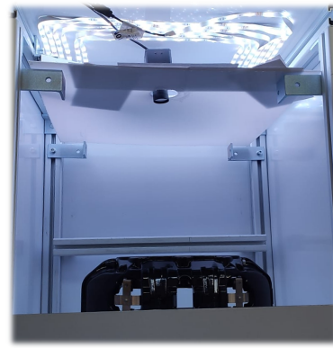
Fig. 3. Image acquisition setup with LED lighting and overhead camera.
