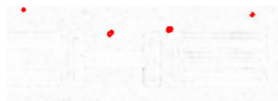
Fig. 8. SSIM map with similarity threshold set to 225/255. All four potential defective areas were detected.
