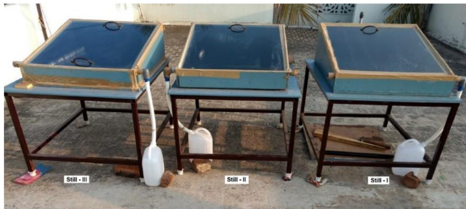
Figure 10. Single slope type of solar still integrated with encapsulated-PCM concentric tube ring [118].
