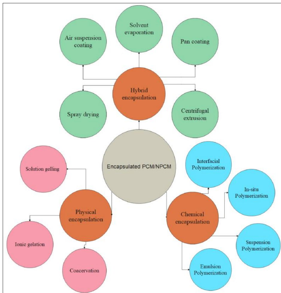
Figure 3. Categorisation of Preparation Methods for Encapsulated Phase Change Materials [5]
