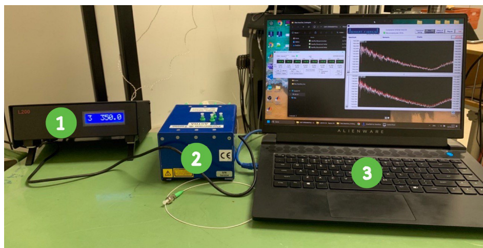
Figure 4. Laboratory setup: (1) thermocouple reader, (2) SmartScan SBI interrogator, (3) control PC.
