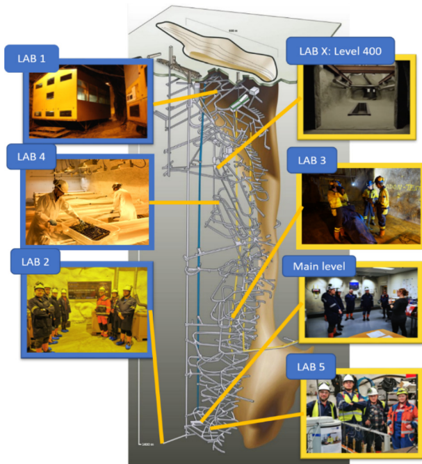
Fig. 27. 3D model of the Callio Lab tunnel network with insets of the various deep underground labs at the mining site.
