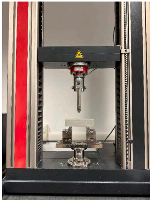
Fig. 4. Flexural strength testing frame.
