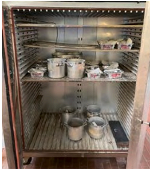
Fig. 3. Part of the samples employed in this study in the oven, placed in appropriate boxes, for the evaluation of dry density.
