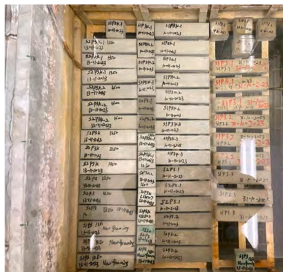
Fig. 2. Water curing of part of the samples.
