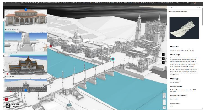
Figure 8. Hybrid solution: a web app dedicated to H-BIM models and their paradata
