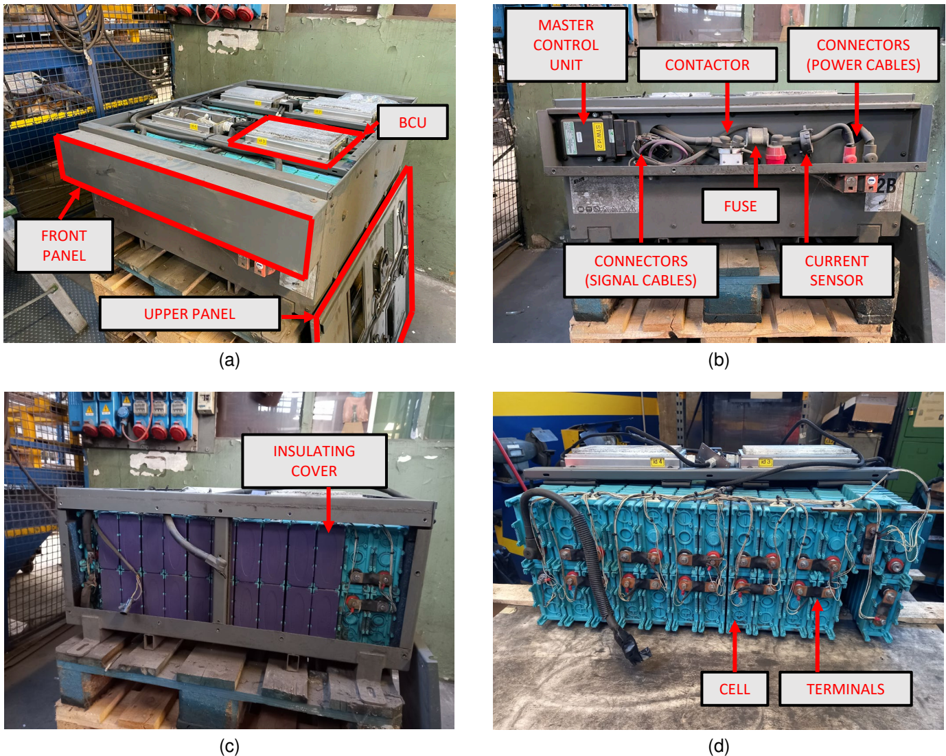
Fig. 4. Case of the battery pack: (a) - just extracted from the vehicle; (b) - front view, after removing the front panel; (c) - front view, after disconnecting the signal and power cables and removing the metallic panel; (d) - interconnected cells managed by the same BCU, extracted from the metallic framework and after removing the purple insulating covers.
