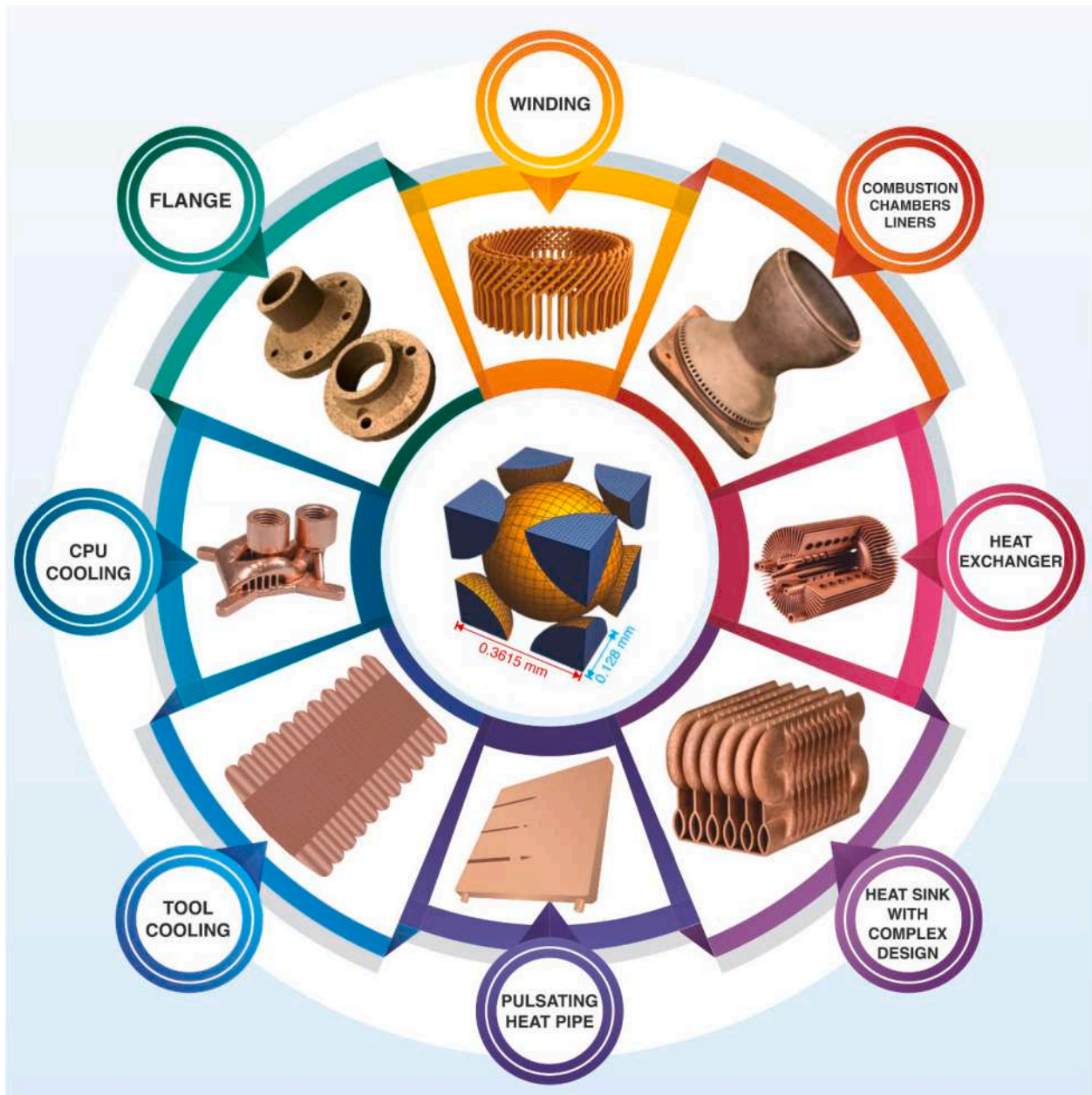
Fig. 4. Potential engineering applications of Cu alloys/composites via additive manufacturing [74–80].
