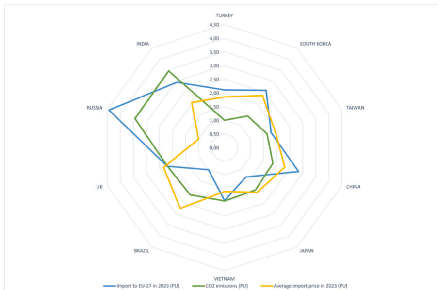
Fig. 4. Per unit evaluation of the CO 2 emitted to produce one ton of HS72 (Turkey as reference), total import to the EU in 2023 (Brazil as reference) and average import price in 2023 (Russia as reference) of the major exporter Countries of iron and steel to the EU.
