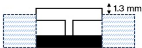
Figure 2. Schematic of the welding setup, including supports to keep the PMMA piece stable and fixed.
