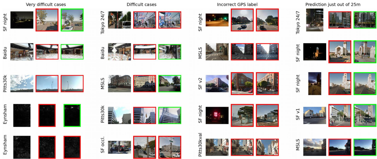
Figure 3. Failure cases, grouped in 4 categories. Each one of the 4 column represent a category of failure cases: for each category we show 5 examples, made of 3 images, namely the query and its top-2 predictions with MegaLoc, which can be in red or green depending if the prediction is correct ( i.e. within 25 meters). The 4 categories that we identified are (1) very difficult cases , which are unlikely to be solved any time soon; (2) difficult cases , which can probably be solved by slightly better models than the current ones or simple post-processing; (3) incorrect GPS labels , which, surprisingly, exist also in Mapillary and Google StreetView data; (4) predictions just out of the 25m threshold , which despite being considered negatives in VPR, are actually useful predictions for real-world applications.
