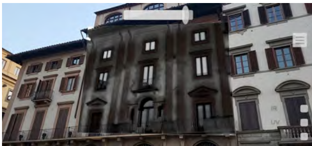
Figure 6. Original triangular peaked facade of San Romolo revealed with thermography in XR app.
