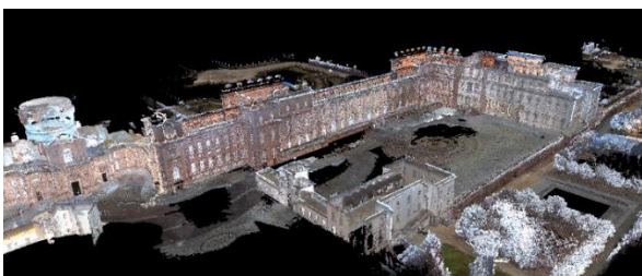
Figure 5: A portion of the registered MMS point cloud on Cyclone Register 360.
