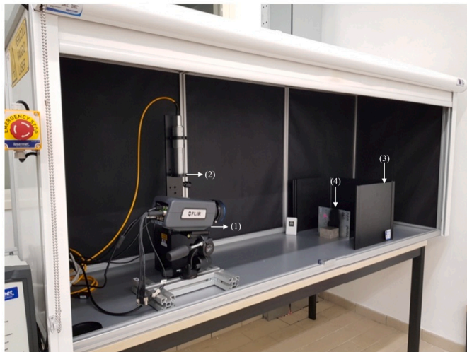
Fig. 3. Active thermography experimental setup with IR camera and laser source. (1) IR camera, (2) Laser, (3) protective panels, (4) test piece.
