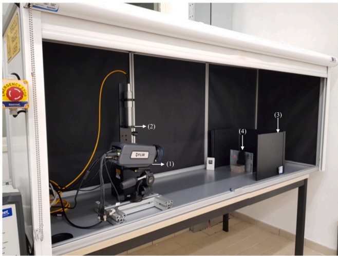
Fig. 3. Active thermography experimental setup with IR camera and laser source. (1) IR camera, (2) Laser, (3) protective panels, (4) test piece.
