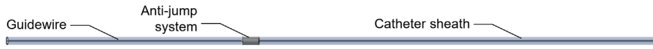
FIGURE 4 | Delivery system including the guidewire, the catheter sheath and the anti-jump system.
