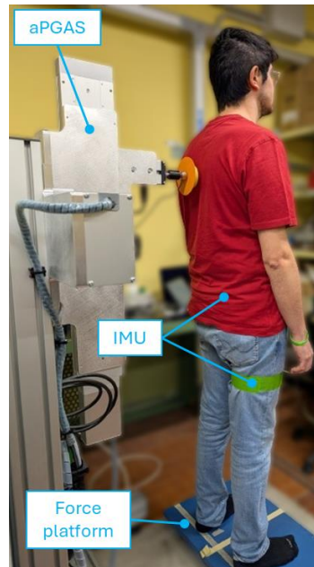
Fig. 2. A dynamic posturographic trial carried out with aPGAS.
