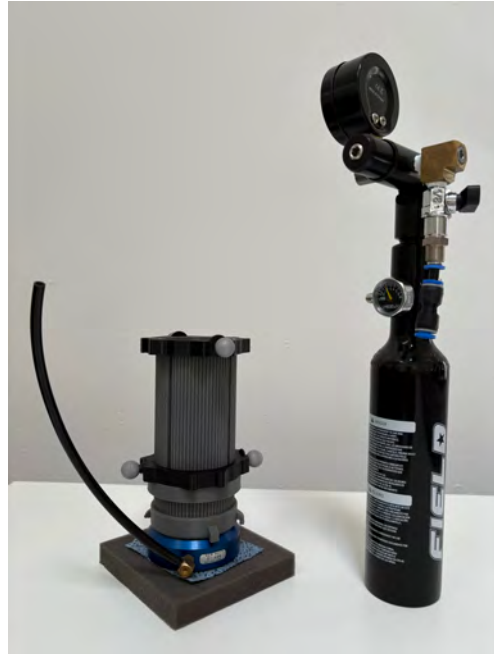
Figure 3. Air tank container with the air bearing laid on a microfibre cloth, reflective markers ( left ), and pneumatic system ( right ).
