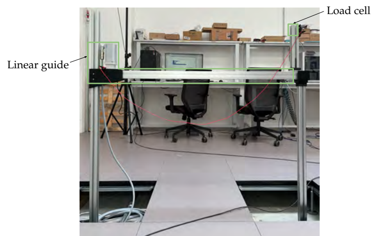
Figure 7. TTS-deployed (static) architecture.
