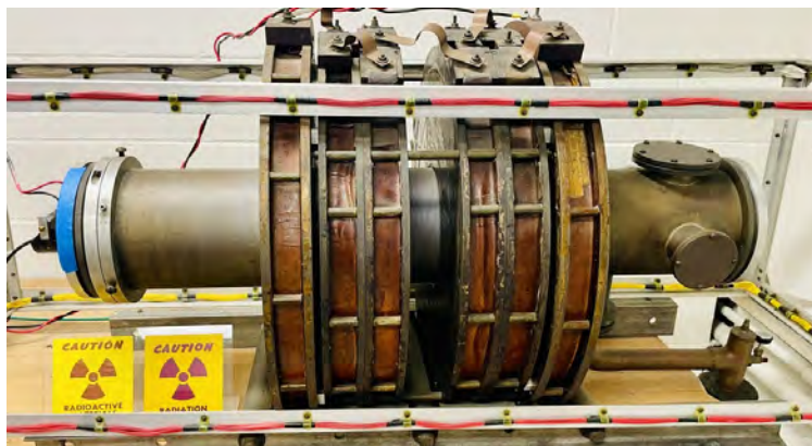
Figure 30. Photograph of the full spectrometer setup used in the experiment. The system includes a vacuum chamber, magnetic lenses, and shielding components arranged to guide and focus electron trajectories for precise beta spectroscopy.
