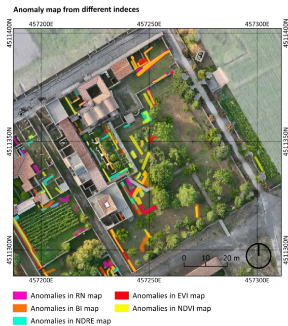
Figure 13: Synthesis of the anomalies detected through the analysis of the five index maps, displayed overlaid on the RGB orthophoto. Each anomaly is represented in a different colour, corresponding to the specific index map in which it was identified, and is shown with partial transparency to facilitate visual overlap and comparison.
