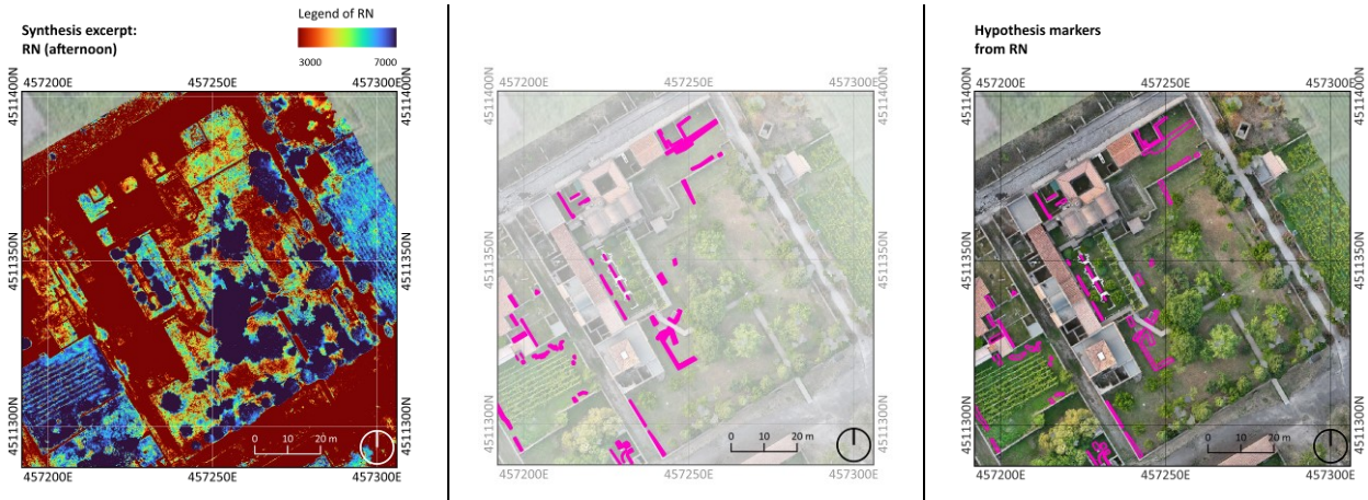
Figure 12: Schematic synthesis of comparison among single index maps (NDVI, EVI 2, NDRE, BI and RN), enhancing in different colours anomalies detected and shown overlapping the optical orthophoto.
