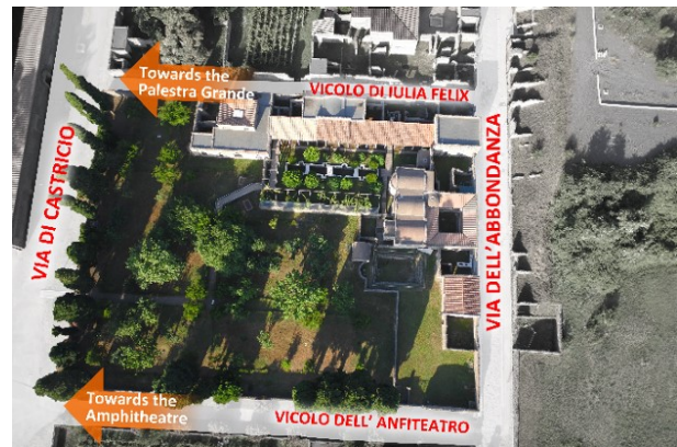
Figure 2: Aerial image of the Praedia of Iulia Felix, highlighting the presence of trees and vegetation that affect flight planning and cast shadows over the area to be surveyed.
