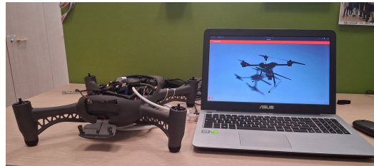
Figure 6. Testbench for Processor-in-the-Loop testing on the UAV's onboard computer.
