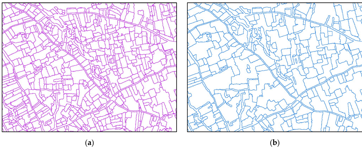
Figure 7. Density of regions obtained by segmenting the PlanetScope NDVI multitemporal dataset with two different combinations of scale level and merge level: in panel (a), the two parameters were set respectively to 10% and 97.5%; in panel (b), they were set to 40% and 97.5%.
