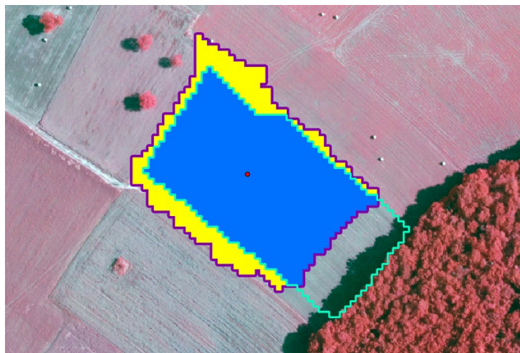
Figure 10. An example of the boundaries of the reference parcel, outlined in aqua green, and the boundaries of the segmented parcel, outlined in purple. The area highlighted in blue represents the overlapping area rate, and the area highlighted in yellow represents the overflowing area rate.
