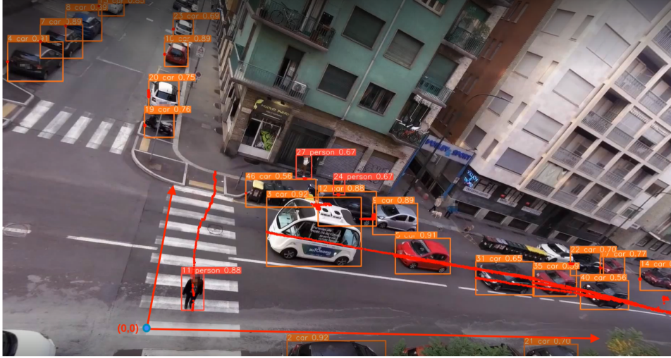
Figure 2: Complete scene with object detection and tracking during a pedestrian crossing in front of the AV.
