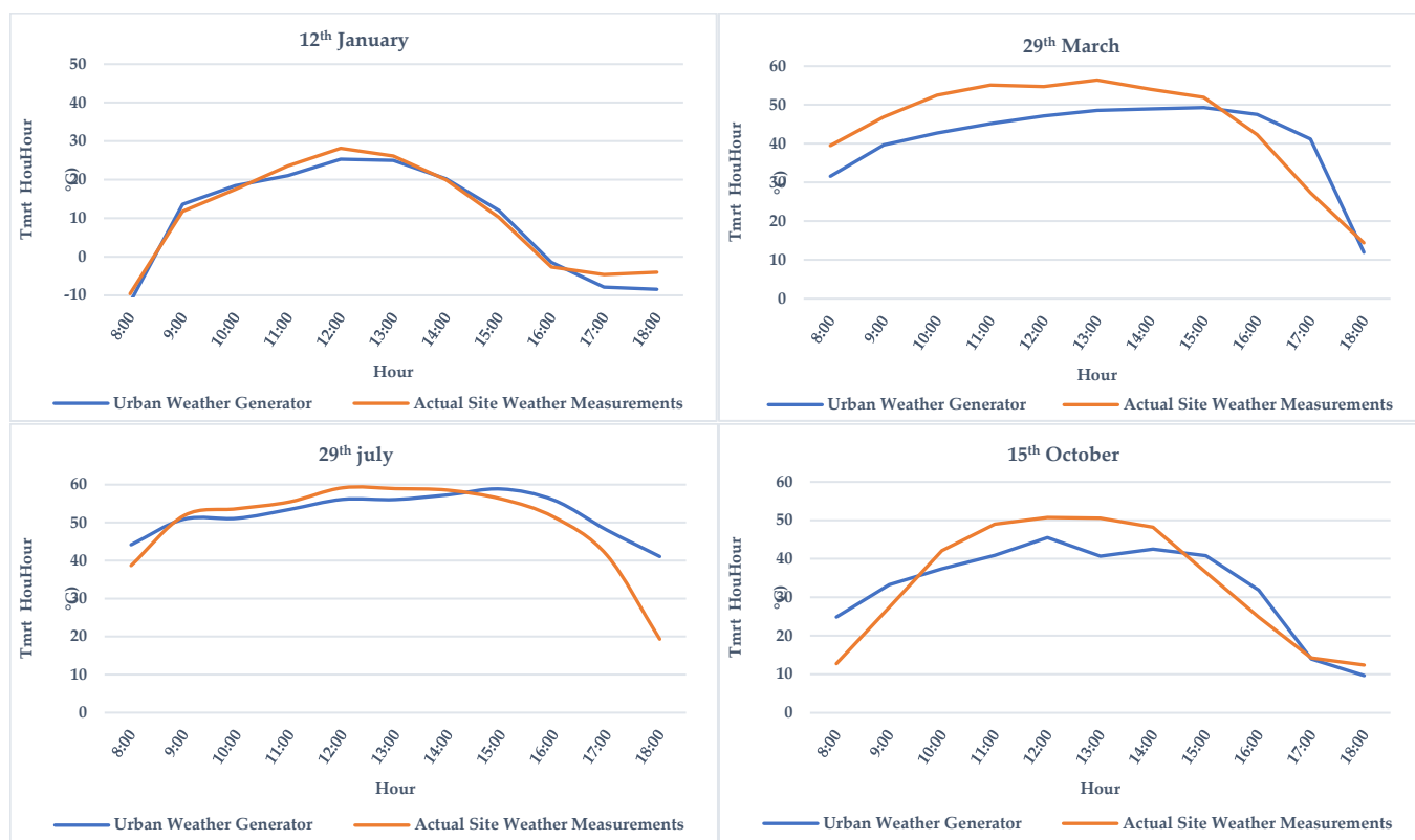
Figure 3. Mean radiant temperature validation.
