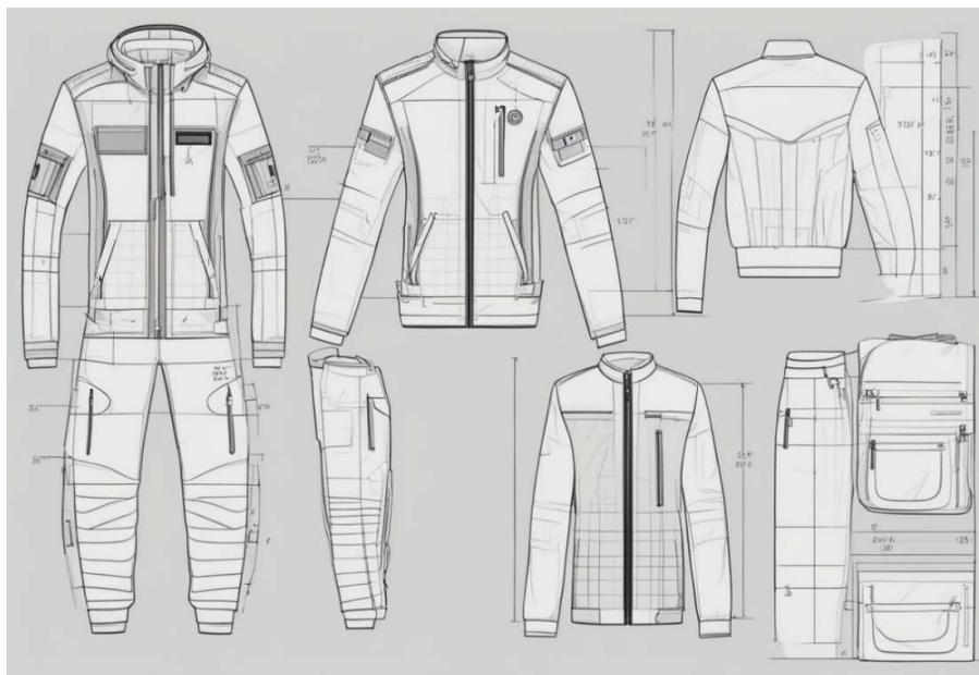
Figure 8. Example of a drawing with associated dimensional specifications for certain types of garments, to support inspectors during inspection. For confidentiality reasons, numerical data are hidden.
