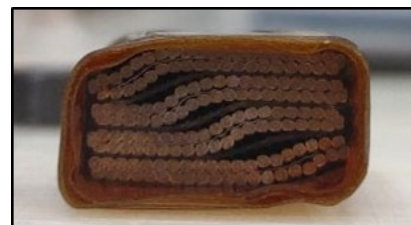
Fig. 5. Buckling failure of the first test specimen.
